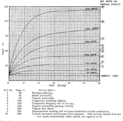
FIG. IV.—TEMPERATURE: TIME CURVES FOR HEATING OF CABLE BY PASSING GIVEN CURRENT THROUGH STEEL ARMOURING
