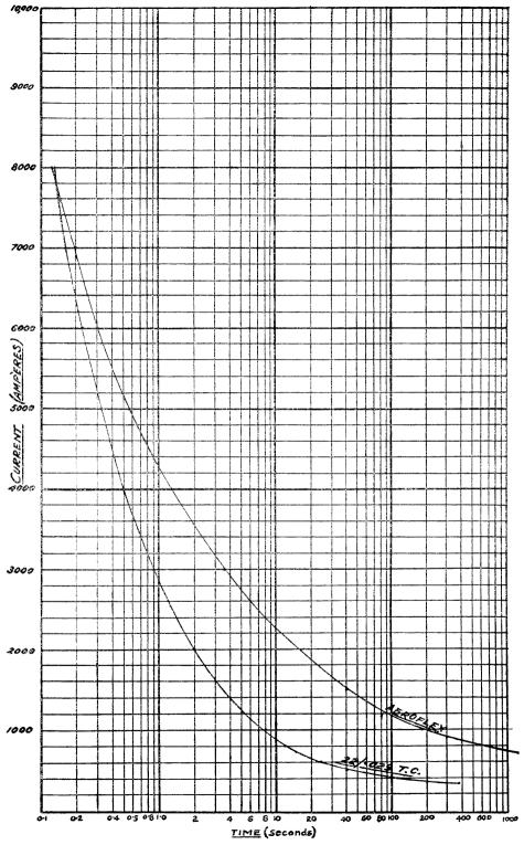
FIG. III.—TIME-CURRENT CURVES FOR AEROFLEX FUSES (500 AMP RATING) LOCATED IN M.E.D. SUBSTATION, LICHPIELD STREET, AND HEAVIEST FUSE (22/·029 T.C.) Used in Services Fuses at Messrs. J. Ballantyne and Co. at Time of Fire
